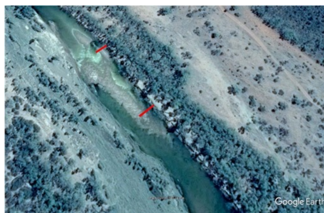
By October 2013, over 15m of the eastern bank had sloughed off, leaving a sediment island in the waterhole. Photo: Google Earth
